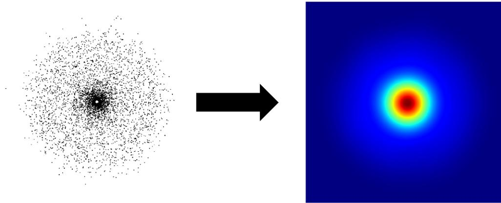
**Figure 3.2. Monte Carlo Impact Points (left) and Associated Probability Density Function (right) Estimated Through Kernel Density Estimation.**
