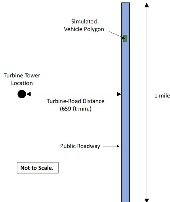
**Figure 4.3. Road Analysis Geometry (figure not to scale).**
