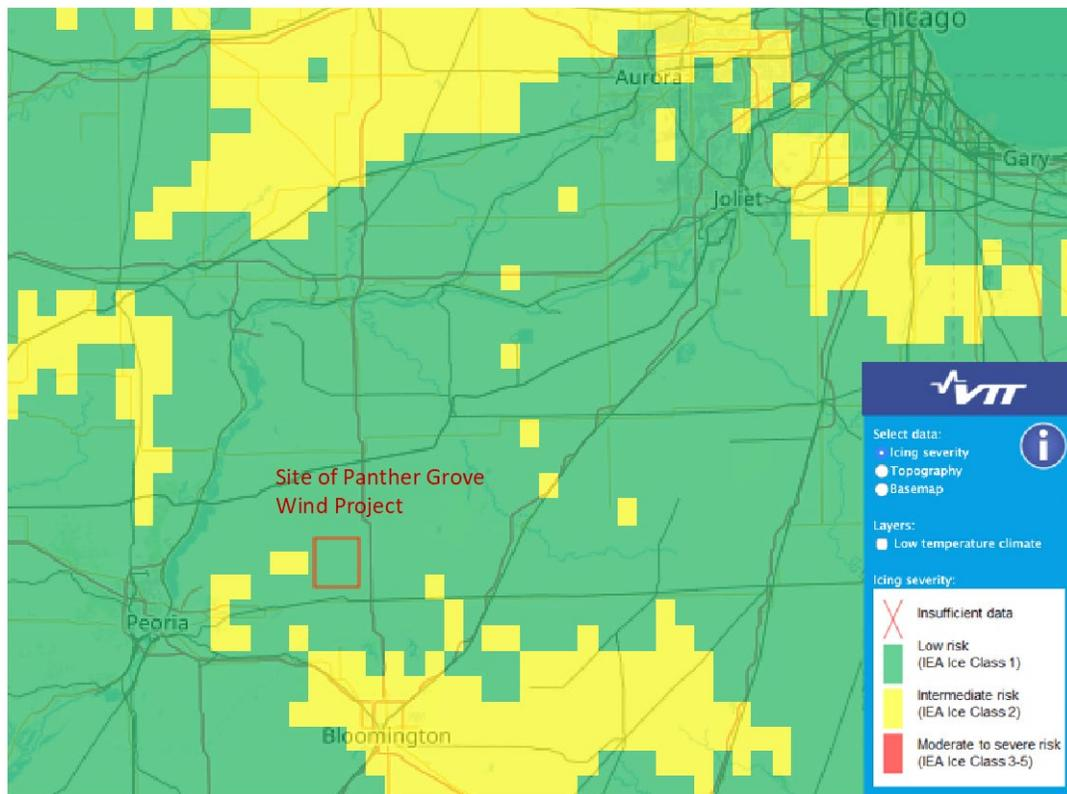
**Figure 1.1. Icing Class Map for Central Illinois [2].**
