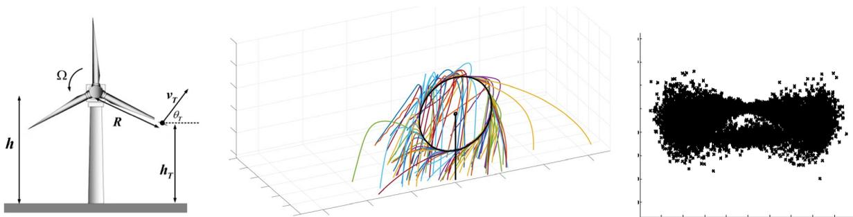
**Figure 3.1. Ice Throw Release Diagram (left), Ice Fragment Trajectories (center), Example Monte Carlo Impact Point Distribution (right).**
