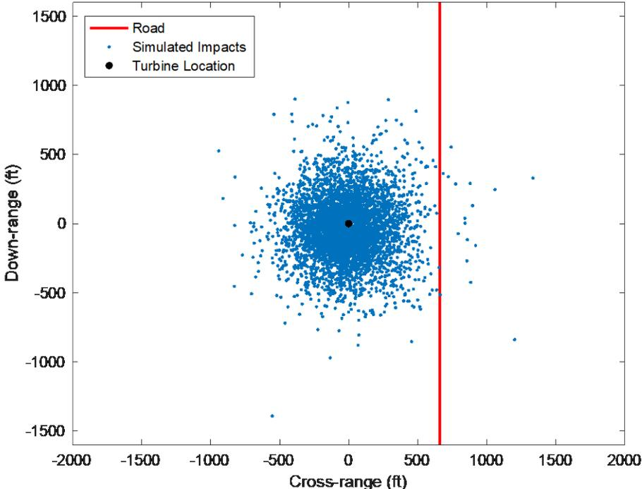
**Figure 4.4. 5,000 Simulated Impacts from GE 5.5/158 Ice Throw and Road Segment at 659 ft Setback.**
